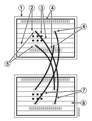
Figure 45. ICL cable connections between two SAN384B chassis
